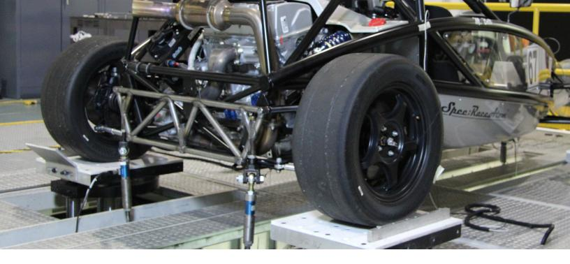
Each of the four wheel platens of the multi-post can produce up to 11,000 pounds (5,000 kg) of dynamic force. Each of the three to four additional downforce actuators can provide up to 4,500 pounds (2,000 kg) of inertial and/or downforce loading. When coupled with 12-inch actuator strokes, the large load capabilities enable a wide variety of road simulations. The wheel platens and downforce actuators are repositionable, allowing for testing of myriad vehicles.
